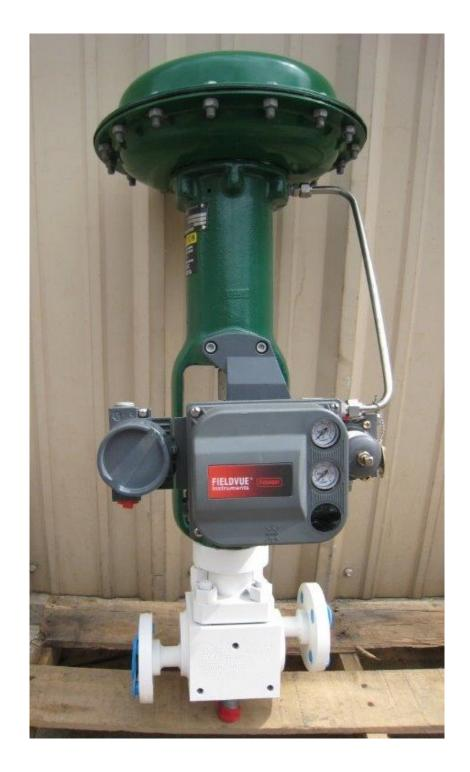
**B.E.L. Valve with Fisher Actuator & Controls**
